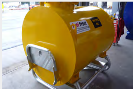
SAFE STEP ACCESS POINT TO MANWAY FILLING POINT
