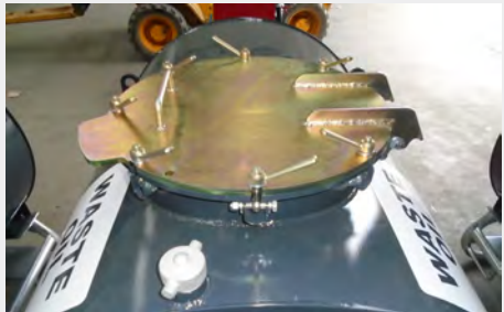
MANWAY FILLING POINT WITH SECURING POINTS AS STANDARD
