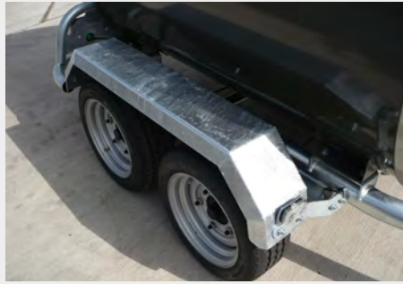
HEAVY-DUTY GALVANISED MUDGUARDS WITH SIDE REFLECTOR AND TRAILER LIGHTING CONNECTION
