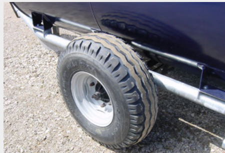
FLOTATION TYRES FOR ROUGH TERRAIN
