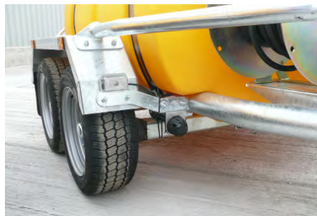
SIDE REFLECTOR AND TRAILER LIGHTING CONNECTION
