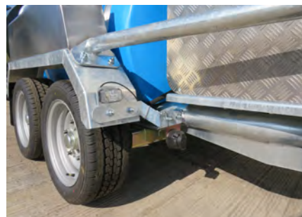
SIDE REFLECTOR AND TRAILER LIGHTING CONNECTION
