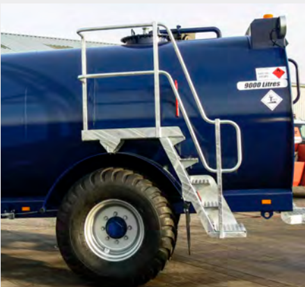
LARGE FLOTATION TYRES FOR OFF-ROAD USE, PLUS GALVANISED REFUELLING PLATFORM (6000 & 9000L)
