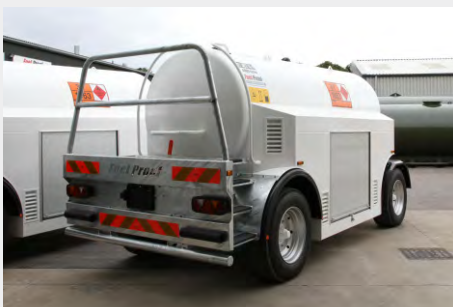
REAR ACCESS STEPS TO MANWAY/ INSPECTION HATCH
