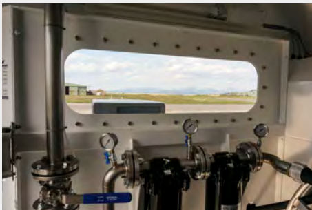
LARGE SIDE CABINET PROVIDES EASY ACCESS TO FUEL DISPENSING EQUIPMENT INCLUDING FILTERS, HOSE/REEL AND OFFSET FILL LINE
