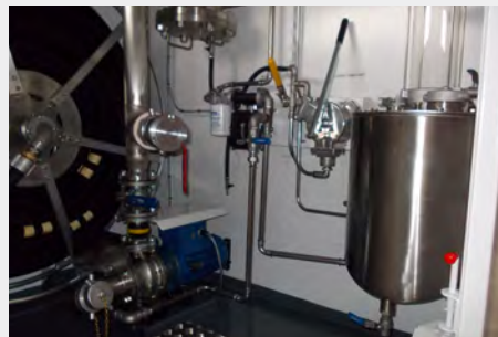
HYDRAULIC HOSE REEL, SELF-LOADING PUMP (OPTIONAL), FILL POINT AND FUEL RECOVERY/SAMPLING SYSTEM
